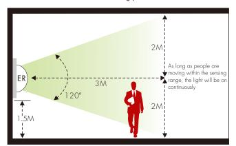
When installing, please pay attention to choosing a proper position and angle, otherwise the sensing distance will be very close or the sensing will be insensitive
