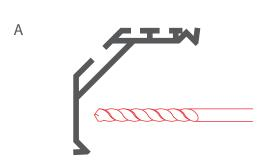
${f 3.}$  Mount the LED strip (D), and slide the spring (E) into the extrusion(A).
