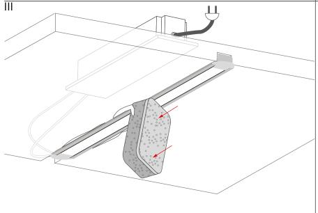
Remove the excess glue from the lighting fixture.
