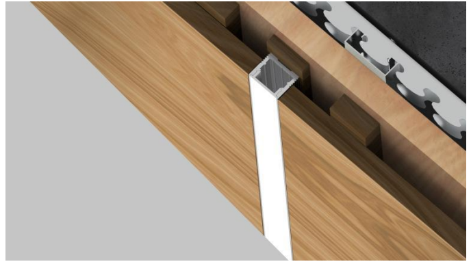
Example of application: wooden decorative board on the wall Cutout:W17*D14mm fixed by glass cement/self-tapping screws
