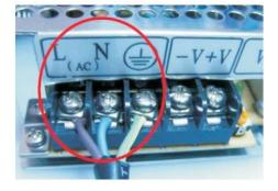
Connect the wires of the power adapter.
