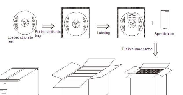
Seal and labeling Seal and put into outer carton
